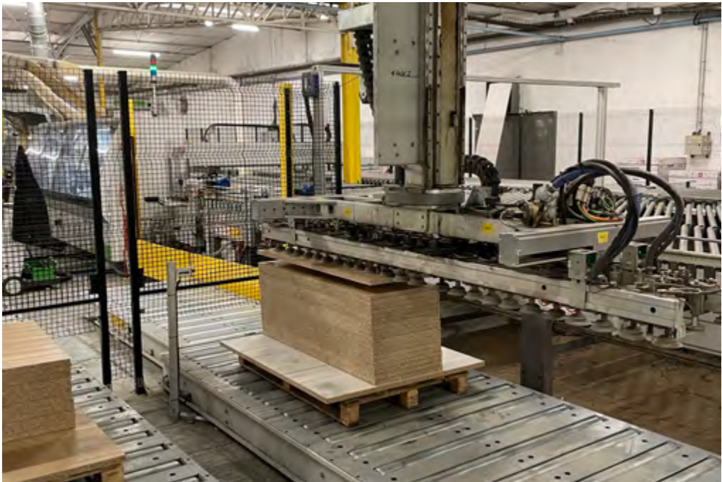
Automatic loading/unloading system used on the worktop edge banding line
